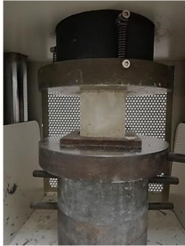
Figure 4. Setup for compression test.
