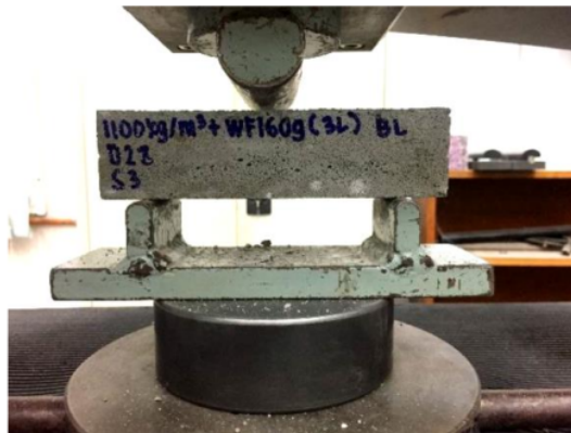
Figure 5. Setup for the flexural test.
