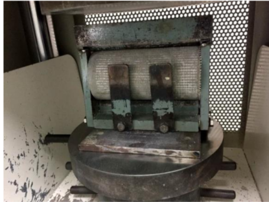
Figure 6. Setup for the splitting tensile test.
