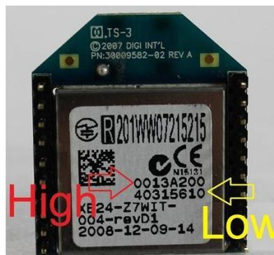
**Gambar 6** *Destination address XBee*
